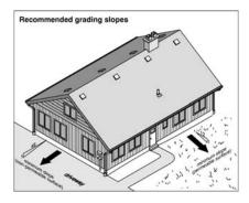
Improper grading around a home can be another factor in a wet basement. Re-grading the exterior landscaping to direct water away from the building rather than towards it, can be another effective solution to moisture problems. Ideally, the ground should slope down and away from the home at a rate of one inch per foot for the first six feet of soil.
