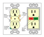
Ground Fault Interrupters are now required in damp locations such as, kitchens/bar countertops, swimming pools, unfinished basements, garages, accessory buildings, crawlspaces and exterior receptacles.
